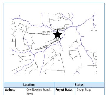
**Description:** This project replaces the Chestnut Avenue Bridge over Newstop Branch and reconstructs the approach roadways. The replacement bridge will be longer, wider and higher than the existing structure. The approach roadways will be modified to reflect the changes to the bridge.
