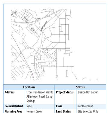
**Description:** Auth Road, Phase II consists of reconstructing Auth Road from the new Metro Access Road to Allentown Road. This project will add capacity, implement geometric improvements, provide for bicycle lanes, resolve storm drainage problems and enhance pedestrian access and safety. Traffic signals, sidewalks, street lighting and landscaping will be installed.
