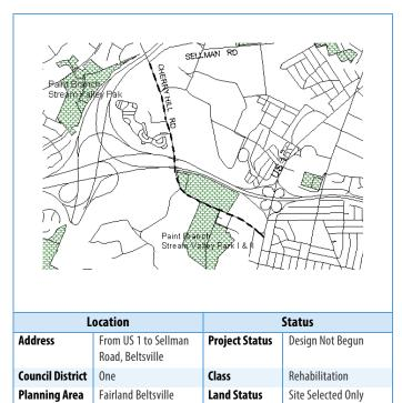
**Description:** This project reconstructs 1.6 miles of Cherry Hill Road from Sellman Road to Little Paint Branch, north of US Route 1, and includes widening two bridges and replacing one. The project will reconstruct the existing two-lane roadway to provide additional traffic lanes. Also included are bike trails, sidewalks, additional traffic signals and street lighting.
