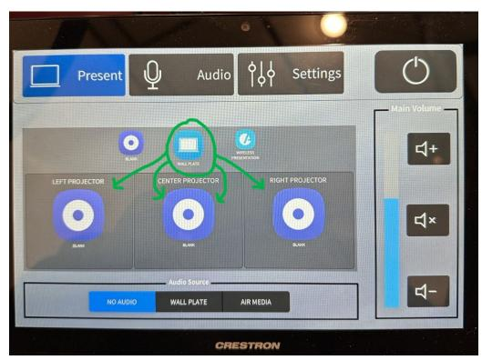
**ALWAYS SHUTDOWN THE SYSTEM!!!** To shut down the system, press the power button on the Crestron control screen. This will shut down all projectors that are powered on.
