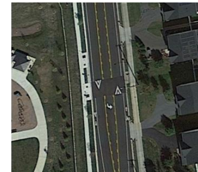
Speed Hump and Bike Lane
