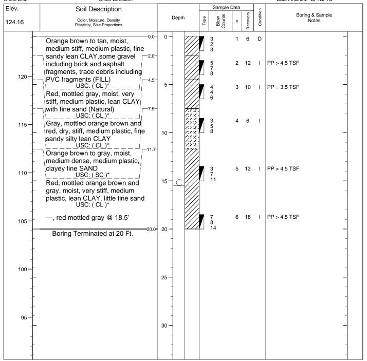
Visual Description - in general accordance with ASTM D 2488 and AASHTO M145 Water Caved Notes: Surface elevations provided by Ben Dyer Associates, Inc. Encountered Dry Dry Completion 17.5' On On 5/19 15.5' Dry
