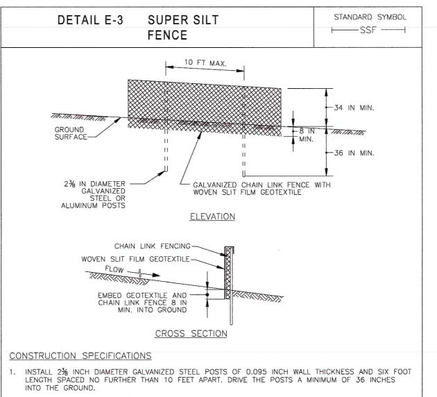
FASTEN 9 GAUGE OR HEAVIER GALVANIZED CHAIN LINK FENCE (2% INCH MAXIMUM OPENING) 42 INCHES IN HEIGHT SECURELY TO THE FENCE POSTS WITH WIRE TIES OR HUG RINGS. 5. FASTEN WOVEN SLIT FILM GEOTEXTILE AS SPECIFIED IN SECTION H-1 MATERIALS, SECURELY TO THE UPSLOPE SIDE OF CHAIN LINK FENCE WITH TIES SPACED EVERY 24 INCHES AT THE TOP AND MID SECTION. EMBED GEOTEXTILE AND CHAIN LINK FENCE A MINIMUM OF 8 INCHES INTO THE GROUND.
