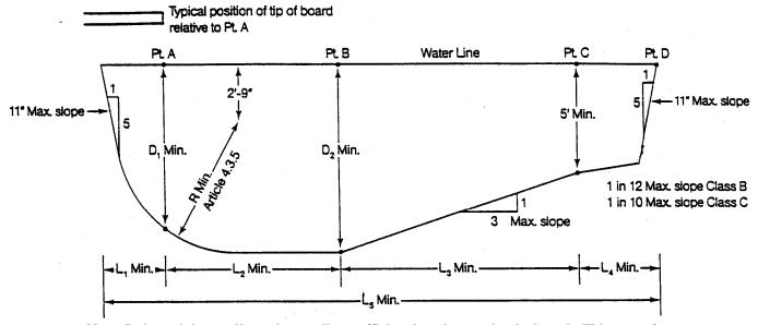
Note:  $L_4$  is a minimum dimension to allow sufficient length opposite the board. This may of course be lengthened to form the shallow of the pool.
