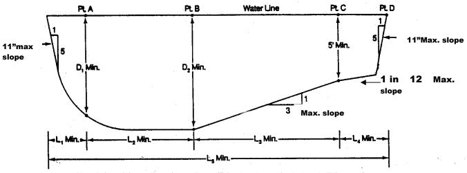
Note:  $L_4$  is a minimum dimension to allow sufficient length opposite the board. This may of course be lengthened to form the shallow of the pool
