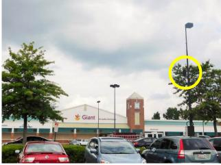
This type of antenna is generally placed on existing light poles, building facades, or other similar short structures capable of supporting the antennas and the small equipment box mounted below the antennas. In most cases these antennas are capable of covering an area less than one-quarter mile in diameter. (By comparison, a typical cell site with a full array of antennas services an area approximately one to two miles in diameter.)
