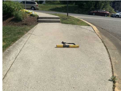
Figure 11 Measurement of Curb Ramp Slopes
