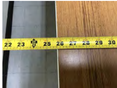
Figure 2 Minimum Clear Width for Two Wheelchairs
